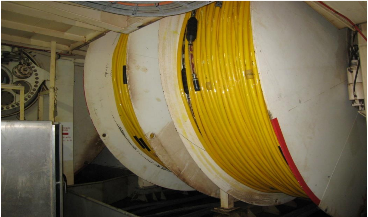
Figure 2-11: Typical seismic streamers
